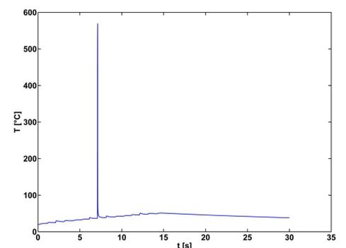
Fig 6 Time temperature curve of the central weld spot (encircled spot Fig 4).
