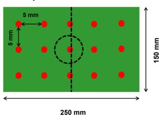
Fig 4 Sketch of the simulated structure; red points indicate weld spots.
