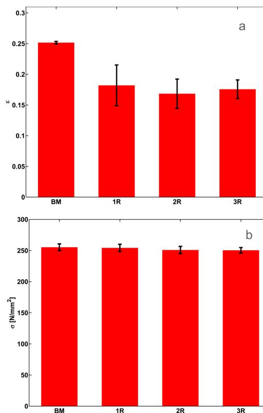
Fig 2. Histograms of the ultimate strain (a) and ultimate stress (b) of the different pin configurations (1R – 3R) and the unaffected base material (BM).
