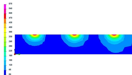
Fig 5 Simulated temperature distribution of the central cross section (dashed line in Fig 4). The depicted temperature field represents the maximum temperature at each node during the computation. The welding order in time was from left to right.
