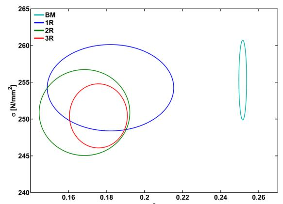
Fig 3. Graphical summary of the ultimate tensile (ordinate) stresses and fracture strains (abscissa).
