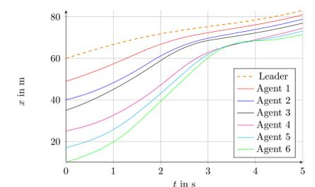
Time-delays and packet dropouts degrade the performance and can cause collisions! Moreover, large initial spacing errors can not be handled.
