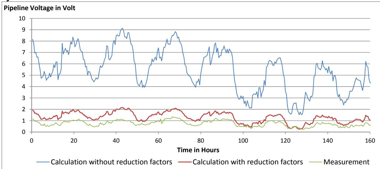
Figure 21 shows an example where the first calculation, without the reduction effect, is much lower than conducted measurements. In this case, there is no reduction effect but an amplifying effect. Investigations in this measurement location finally showed that the specific soil resistivity was substantially higher than in the surrounding area, whereof the value for the calculation was based and led to incorrect results.
