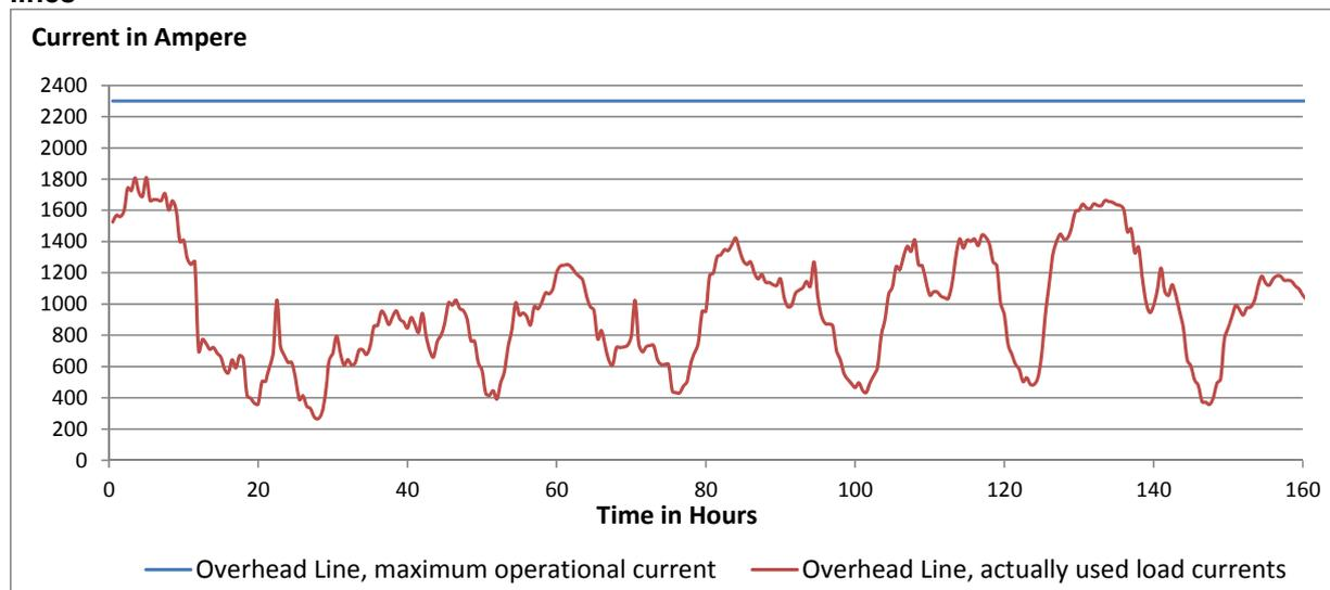
**Figure 4: Difference between maximum operational currents and load currents for railroad systems**
