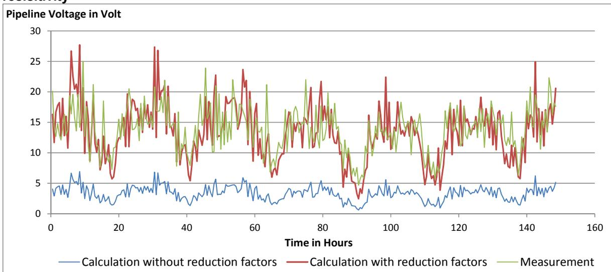
Even with knowledge of all known parameters, there exist some examples where the difference between measurements and calculations can range from “low” to “unacceptably high”, see Figure 22. Possible factors can be unnoticed connected earthing systems which reduce the pipeline voltage in this location, measurement errors or other unknown factors.
