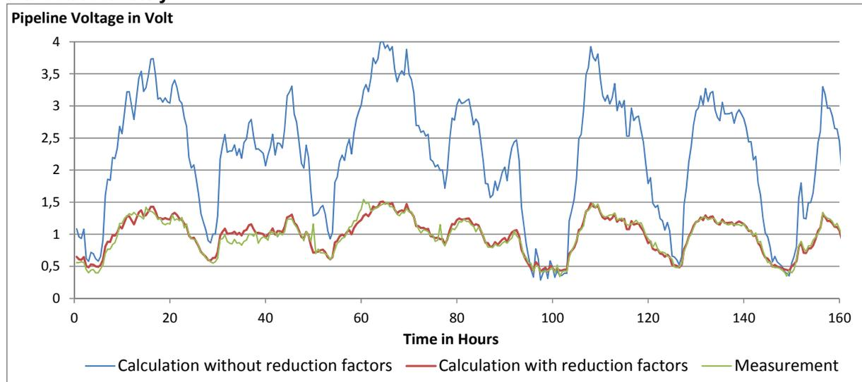
**Figure 19: Pipeline voltage calculation versus measurement, location 5, parallel pipeline with high soil resistivity**
