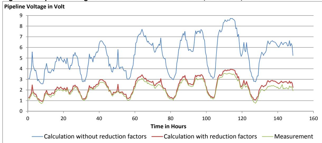
**Figure 17: Pipeline voltage calculation versus measurement, location 3, railway**
