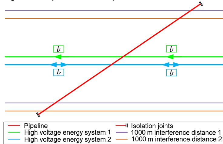
If both HVESs are situated close to each other, the coupling effect has to be considered. This can be realized using the node admittance matrix.
