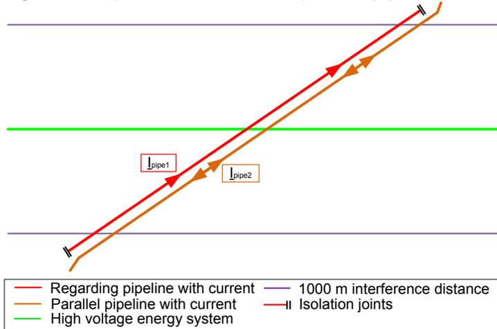
The degree of the parallel pipeline reduction effect depends mainly on the pipeline diameter ratio. For example, is the parallel pipeline diameter smaller, the effect on the regarding pipeline is substantially smaller with the effect of a much smaller parallel pipeline reduction effect.
