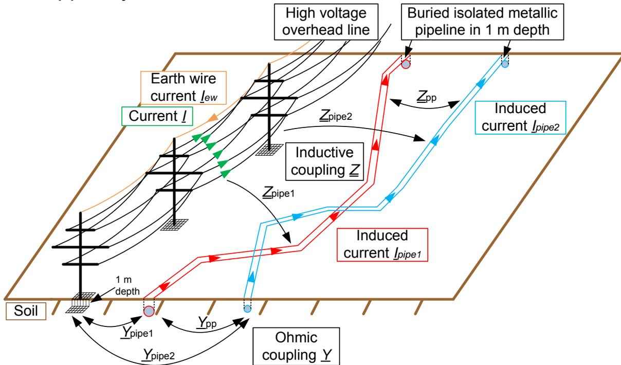
In this configuration, the same mathematical description from the GES calculation in Chapter 3.2.1 is valid, as long as different calculation parameters are considered. The coupling  $Z_{pp}$  exists because for the respective pipeline, the other pipeline is again an active energy system with its own magnetic field, caused by the additional current ( $I_{pipe1}$  or  $I_{pipe2}$ ) arising from the inductive interference of the HVES.
