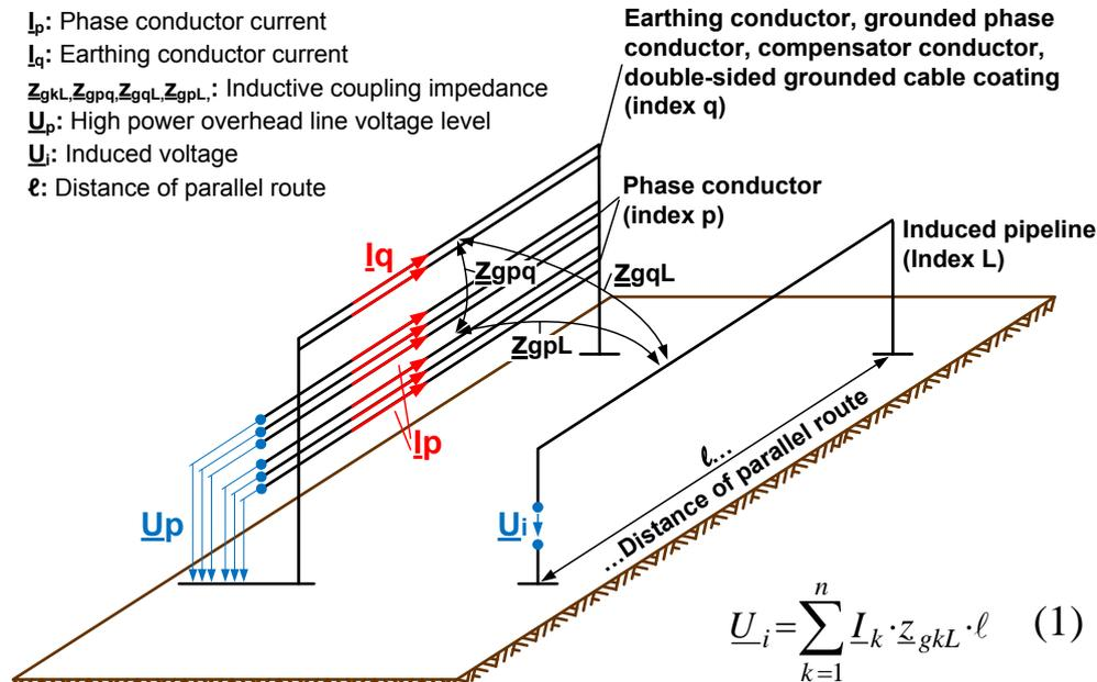
Figure 1 shows the inductive interference between an interfered pipeline and an interfering two-circuit high voltage overhead line. The phase conductor current  $I_p$  is set by the current for normal operations and short-circuit-situations, all other currents  $I_q$  flow through other conductors and cable coatings. The following matrix (2) leads to the currents  $I_q$  (3).
