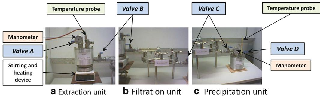
**Fig. 1** Experimental set-up for extraction of *scl*-PHA under high temperature and pressure conditions using the “*scl*-PHA anti-solvent” acetone. The apparatus consists of an extraction unit (a), a filtration unit (b) and a precipitation unit (c). Valve A serves for inlet of nitrogen to generate an oxygen-free atmosphere
