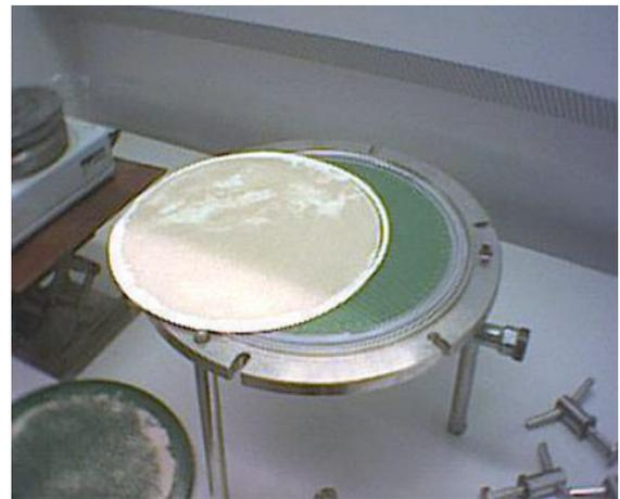
**Fig. 2** Internal of the “Filtration unit” FU after reassembling. Retained NPCM is visible on the filter paper
