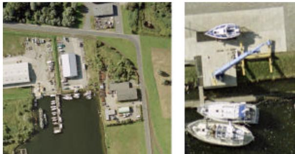
Figure 7: Aerial image taken at a scale 1:5000. The AGFA X100 color negative film shows a remarkably fine granularity and allows scanning at a resolution of 2500 dpi.
