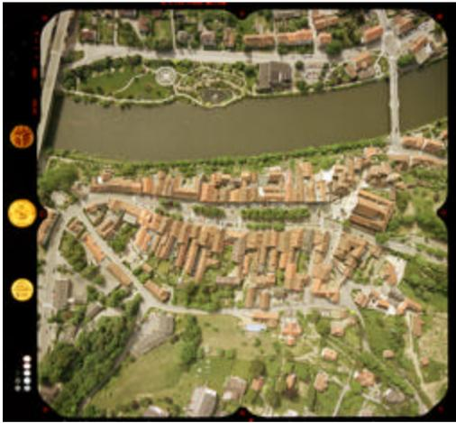
Figure 2: An aerial image, 23 cm by 23 cm, results in a digital file of several hundred megabyte of data (e.g. 705 MByte @ 15  $\mu$ m pixel size and 3 by 8 bit color depth)
