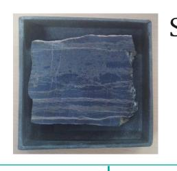
Sample crushing and leaching in 3 M HNO<sub>3</sub> at 70°C for 24 hours to capture both phosphate and carbonate phases.
