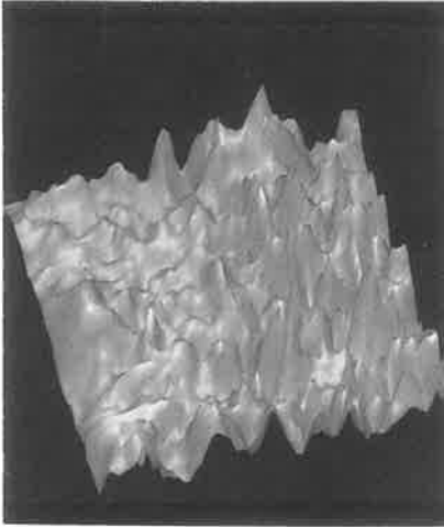
Figure 15. Difference DEM produced by taking the absolute values of the differences in height at each point of the two DEMs in Fig. 14. The r.m.s. difference is \pm 100 m. Note the high frequency of the errors.
