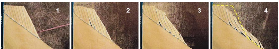
Fig. 4 Multiple block slumping.
