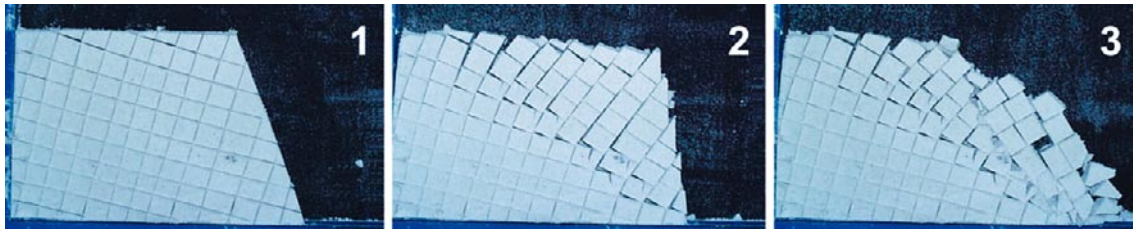
Fig. 7 Toppling of a blocky rock mass.
