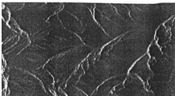
Fig. 2. A 1805 \times 973 pixels ERS-1 sub-scene of Otztal, Tyrol. The image was acquired during an ascending orbit with a look angle of 23 deg. The area shown covers approximately 22 km x 12 km, pixel size is 25 m x 25 m. Copyright esa.
