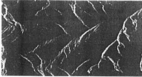
Fig. 4. Presumed layover areas extracted from Fig. 2 by thresholding. The threshold value was determined automatically from the percentage of layover pixels in Fig. 3.
