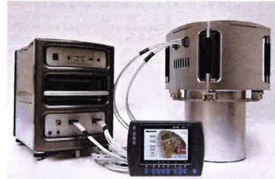
Fig. 7.3-2 The UltraCamX digital aerial camera system with the Sensor Unit (right) and the airborne Computing Unit including two removable Data Units (left). The camera is operated in the air through the Interface Panel (middle)
