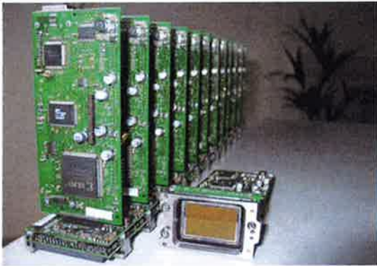
Fig. 7.3-6 Full set of 13 UltraCam CCD-sensor and electronics components. Nine units are used for the large-format panchromatic image; four units are responsible for the multispectral bands
