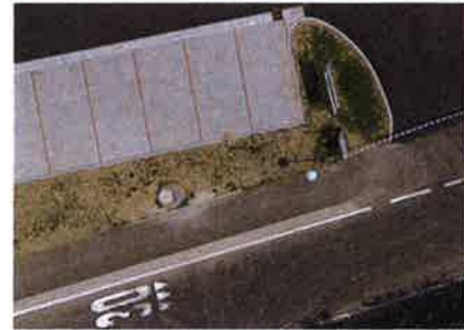
Fig. 7.3-1 Large scale aerial image at 3 cm GSD. This 700 pixel by 500 pixel sub-area of an UltraCam image covers only 21 m by 15 m on the ground
