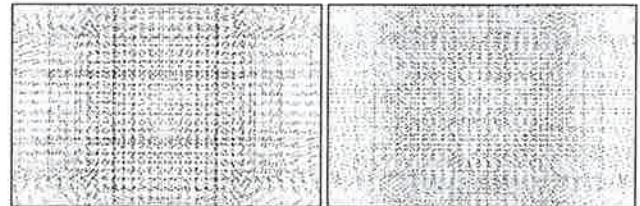
Fig. 7.3-11 The automatically detected image positions cover the entire frame of the camera. About 18,500 points are detected in the panchromatic channel (left) and 17,500 points are detected in each of the four colour bands (right). A single image trigger will therefore produce a total of about 90,000 points
