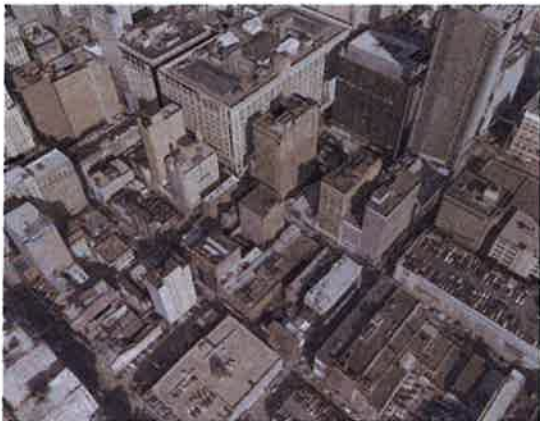
Fig. 7.3-19 3D model of Philadelphia, automatically computed from UltraCam images with large overlaps. The photo texture of the 3D scene was also extracted from UltraCam images
