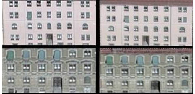
Figure 3: The marked sections of Figure 4 have been rectified. At left are two sections from the oblique data at  $45^{\circ}$ , at right from the vertical data at  $27^{\circ}$ .
