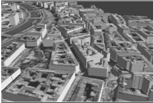
Figure 5.1 Draping the photo texture over the 3D geometry (above) can support quality control, and result in a product that presents the material properties at each surface by means of the gray values of a photograph (below).
