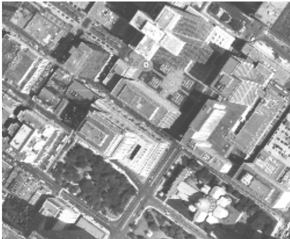
Figure 6.1: Segment of photo coverage at resolution of 0.9 m per pixel, simulating a high resolution optical space image. It should be possible to extract commercial buildings from such imagery.
