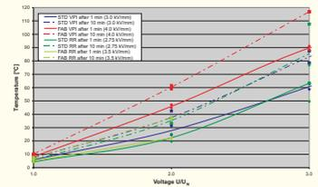
Figure 5: Warming-up of voltage grading tape
