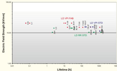
Figure 7: Life time points of VPI and RR bars produced with different mica types
