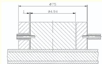
Figure 2: Test-setup Capacitance and  $\epsilon_r$  Measurement
