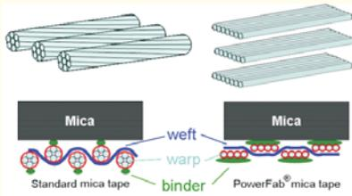
Figure 1: Schematic design of glass yarn
