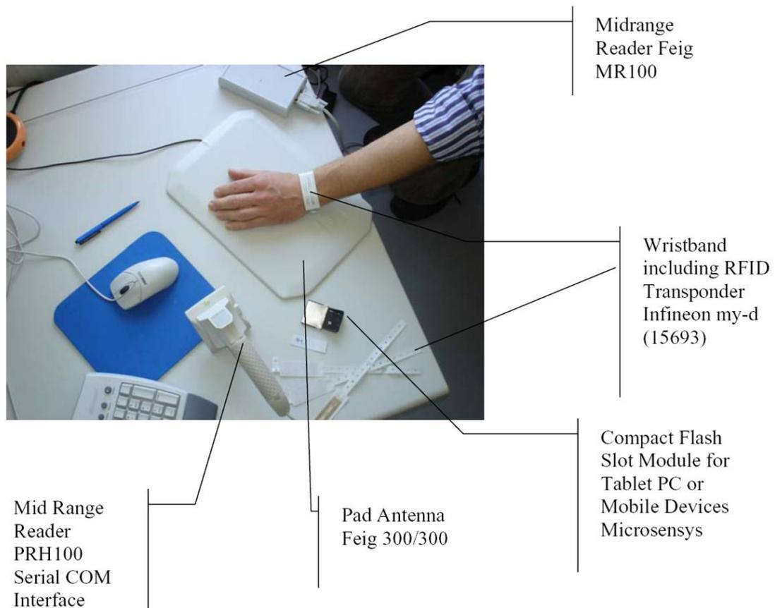
Figure 1: Devices used during our first experiments
