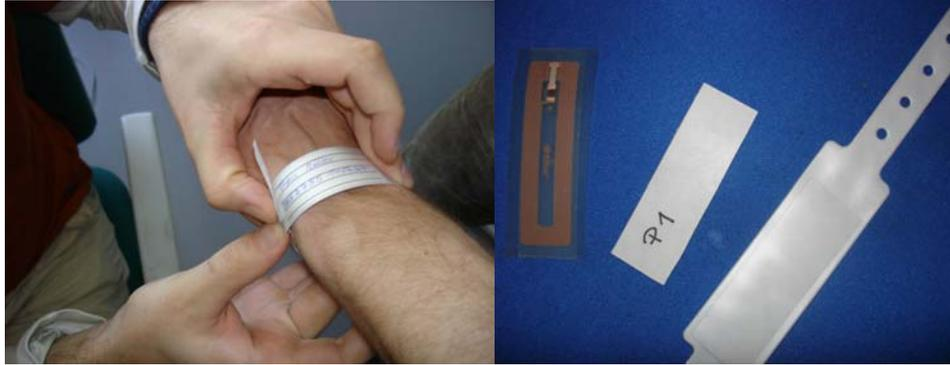
Figure 3: Inside the standard wristband an RFID tag (right) is added
