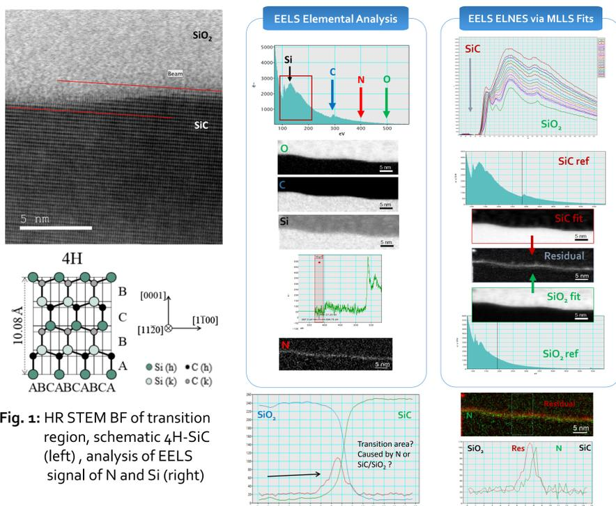
**Fig. 1:** HR STEM BF of transition region, schematic 4H-SiC (left), analysis of EELS signal of N and Si (right)
