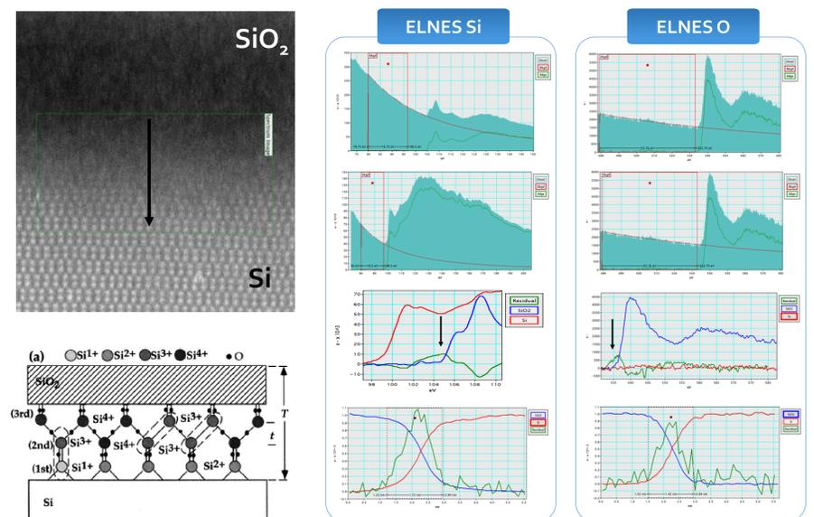
**Fig.2:** HR STEM HAADF of transition region, schematic of transition [1] (left) Analysis of ELNES signal of Si and O (right)
