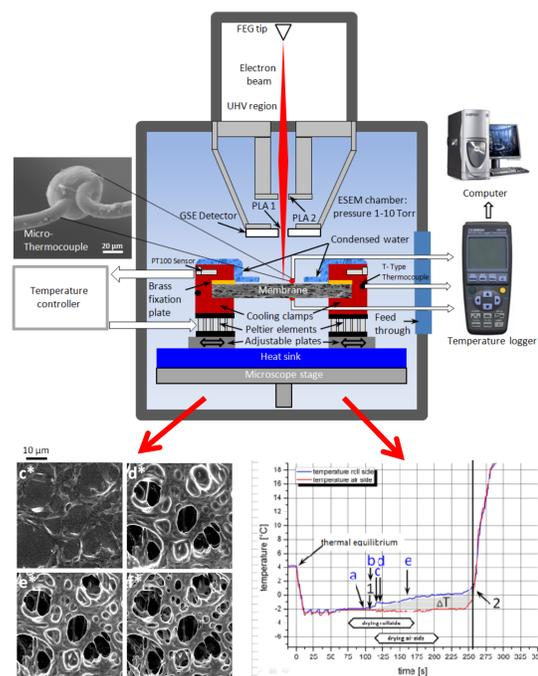
Fig. 3. Top: schematic of the experimental setup; bottom left: Drying of the surface pores as a function of the drying time; bottom right: the temperatures at both membrane surfaces of the cooled membrane (4°C) as a function of the drying time.
