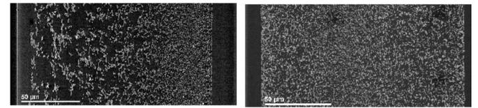
Fig. 1. SEM images (BSE) of the cross sections of two polyethersulfone based membranes: Membrana DuraPES®450 (left) and Sartorius 15406 (right).
