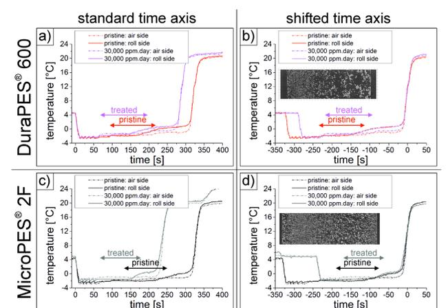
Fig. 4: Temperature profiles of 2 different membranes before and after treatment with a dose of 30,000 ppm.day NaClO with a concentration of 30,000 ppm. The double arrows indicate the start and end of the drying of the surface pores at the air side. Two time axes were used for a better visualisation of the drying behaviour of the membranes. The double arrows mark the start and end of the drying of the surface pores. The insets show a cross section of the respective membrane.
