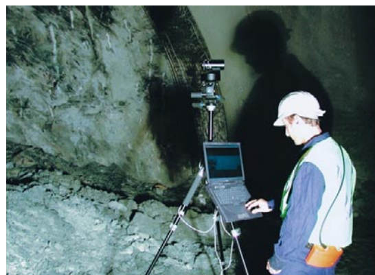
Fig. 2 The imaging system applied in a subsurface environment.
