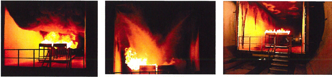
Figure 12: Images from test #14 with HPWMS, w/o activation (left), with activation (middle), activation turned off (right)
