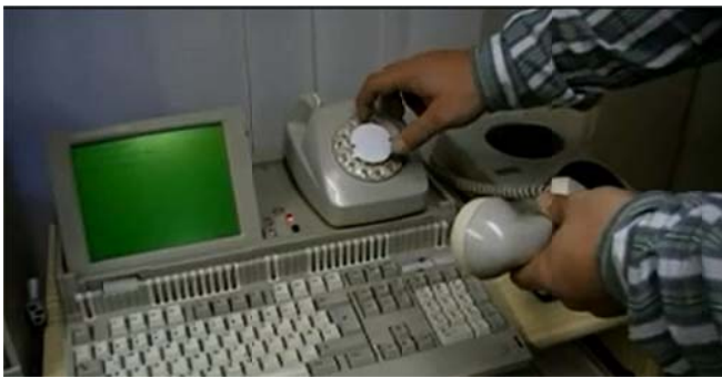
Figure 2: Acoustic coupling of two computers via a telephone line - www.youtube.com/watch?v=ychSsyn4xPs .
