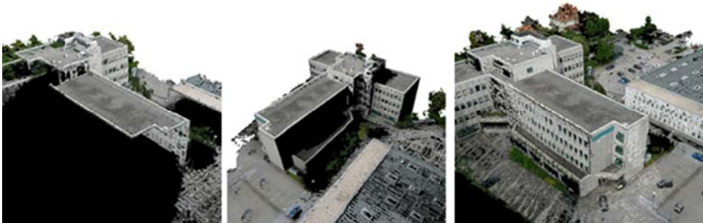
Figure 12 : Point clouds from two separate sets of MAV-based image blocks [left and middle] of one terrain object. These point clouds get fused into a single point cloud to the right [from Wendel et al., 2012]
