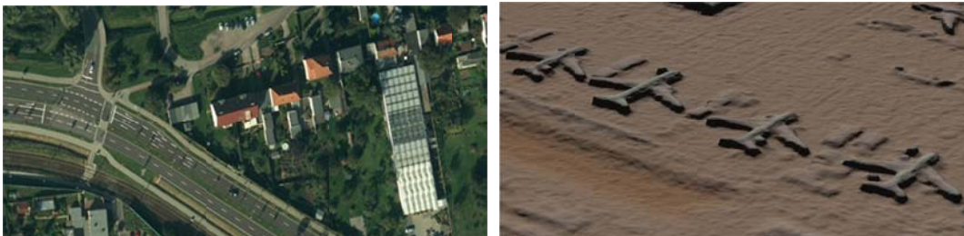
Figure 8: Global Ortho Photo at a pixel size of 30 cm [left] and DEM with postings at 1 m interval [right]. [Walcher et al., 2012].
