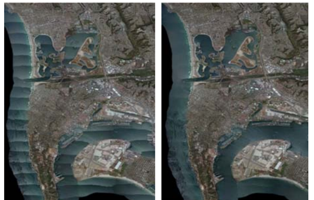
Figure 13a: Specular reflection on water near San Diego, CA, affecting each individual photo and flight line
