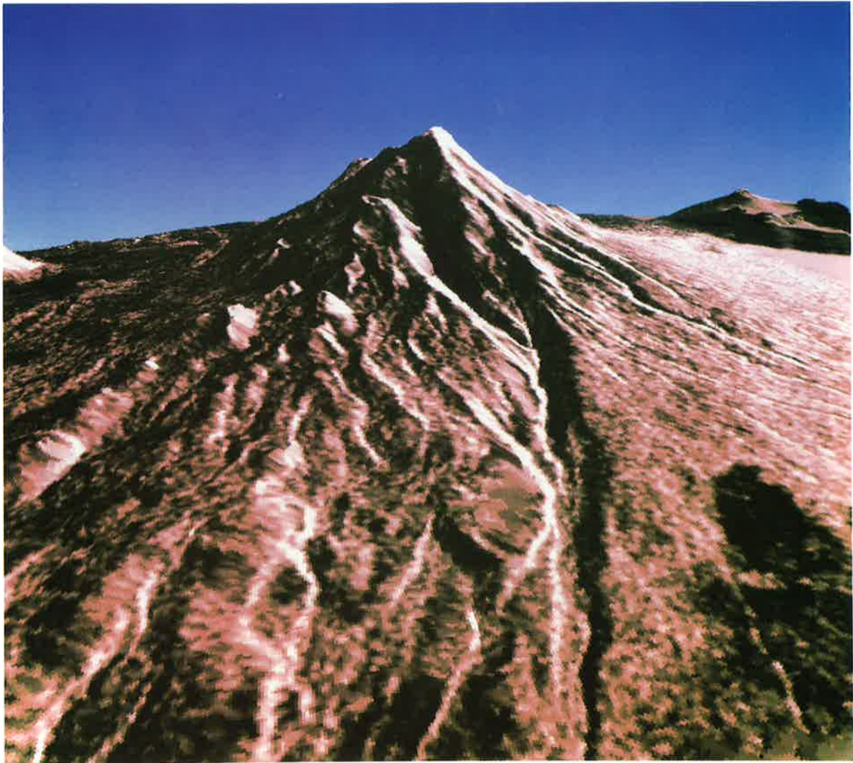
Fig. 7. Perspective view of the radar derived DEM, with radar image brightness superimposed and coded as color.
