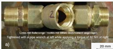
Figs. 12a and b: a) Angular-seated valve 2 with thread nipples, non-fixed. Left side: Octagon, tapered, with no hemp used; Right: Hexagon, cylindrical, with 0.05 g of hemp; b) condition after 72 h 5% ammonia test, cleaned in an alcohol ultrasonic bath
