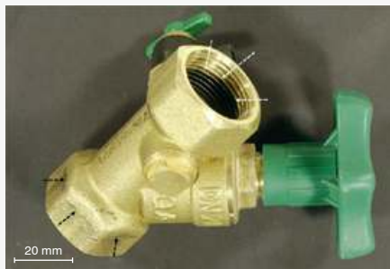
Fig. 1: An inclined-seat valve with inflow-sided cracks on the threaded socket (black arrows). The white arrow marks the length of thread engagement on the outflow side.
