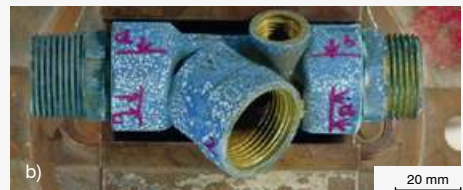
Figs. 12a and b: a) Angular-seated valve 2 with thread nipples, non-fixed. Left side: Octagon, tapered, with no hemp used; Right: Hexagon, cylindrical, with 0.05 g of hemp; b) condition after 72 h 5% ammonia test, cleaned in an alcohol ultrasonic bath
