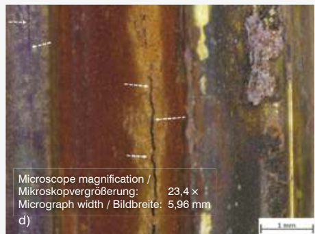
Figs. 2a to d: Inflow-sided thread in the region of thread engagement length: a) and b) cracking along the inside thread diameter; c) and d) detailed micrographs
