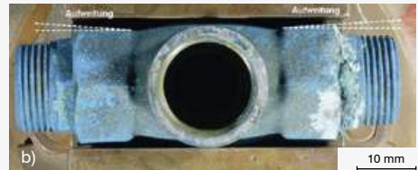
Figs. 14a and b: a) Straight-seated valve 3 with cylindrical thread nipples / no hemp used at left, 0.2 g hemp used at right; b) condition after 144 h 5% ammonia test and cleaning in alcohol ultrasonic bath
