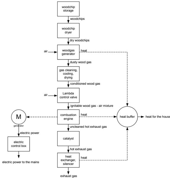
Fig. 1. Functional overview of the cogeneration plant
