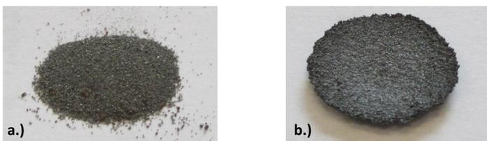
Fig. 1) a.) pure unreacted iron sponge powder b.) sintered iron sponge after two redox cycles at 600 C.
