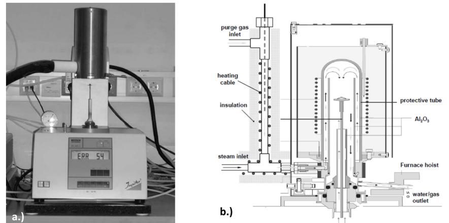
Fig. 3) a) STA449C Jupiter Netzsch . b) schematic gas flows.
