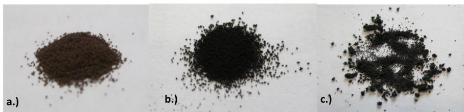
Fig. 2) a.) unreacted 5% sample b.) 5% sample after ten cycles at 750 C c.) 5% sample after ten dynamic cycles.
