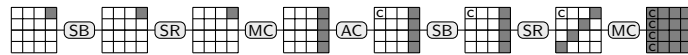
Figure 4.5.: Characteristic for the F -function with 5 active S-boxes. Notation: \square inactive, \blacksquare active, \boxplus internal difference due to round constants
