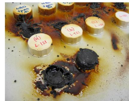
Photograph of cylindrical specimens after self-inclination at room temperature during drying under ambient conditions.
