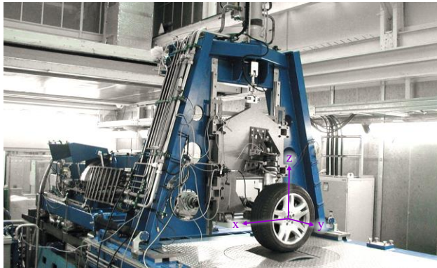
Fig. 4. Drum driven suspension and brake test rig for creep groan parameter matrix experiments, adapted from [14].
