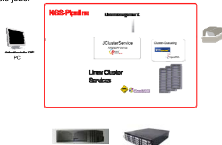
Figure 2: Software & Hardware Architecture The pipeline is based on the Java 2 Enterprise Edition (J2EE) three-tier architecture and uses JClusterService to communicate with the HPC cluster. The currently used hardware architecture consists of two X4600 Sun Servers (32 CPUs, 160 GB RAM) attached to SAS storage with 16 TB (and extendable to max. 256 TB) via Gbit Ethernet interconnect.
