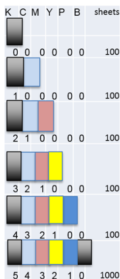
Figure 1. Print trial A. The stack of printed sheets obtained from the trial. The numbers below the colours represent the amount of back-traps of one colour.
