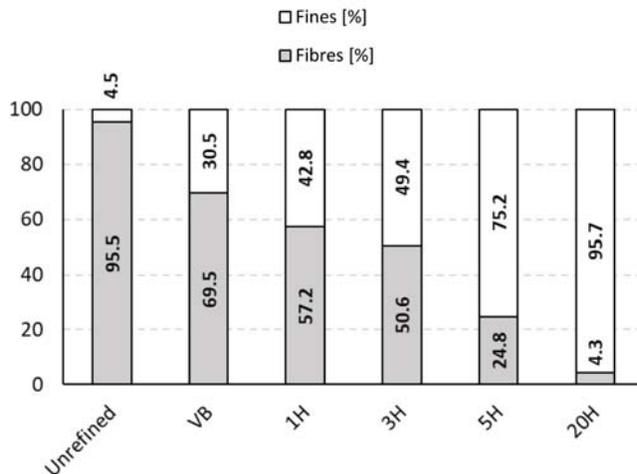
Fig. 3. Fibres (white area) and fines (grey area) fraction measured for VB and the high-pressure homogenized samples according to Tappi T-261 cm-10
