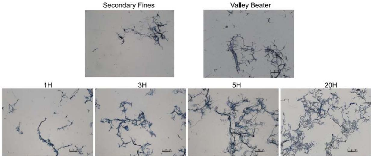
Fig. 4. Microscope images of the different stained fine fibrous materials (scale bar in images is 100 µm)
