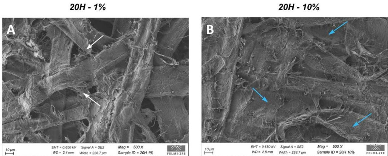
Fig.9. SEM images of handsheets with A) 1% and B) 10% of material 20H (magnification 500x). A) The white arrows indicate zones where fibrils from the added fibrous material act as additional connections between two fibres. B) The blue arrows indicate the areas forming a secondary network of fibrillar elements composed of the added fine fibrous material
