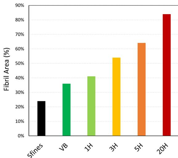
Fig. 5. Result of average fibril area for each fine fibrous material resulting from image analysis of stained microscope samples.
