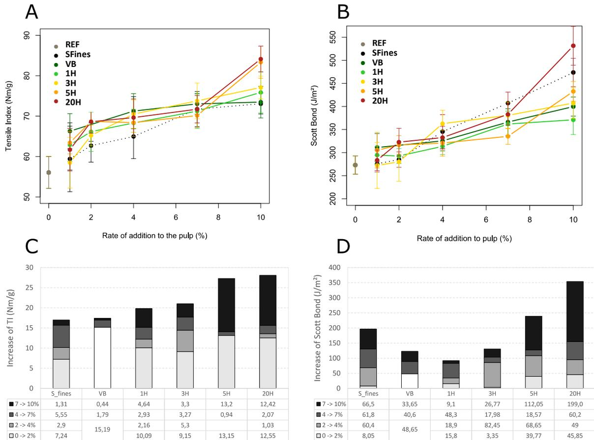
Fig. 7. A) Influence of material type and rate of addition on tensile index (TI); B) Influence of material type and rate of addition on z-strength (Scott Bond); C) Contribution of each successive rate of addition to the increase of TI; D) Contribution of the partial increases of SB for each successive rate of addition
