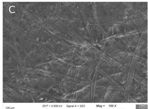
Fig. 6. A) Influence of the type and addition rate of the different fine materials on air permeability of handsheets B) and C) SEM images of surfaces of handsheets produced with (B) 1% and (C) 10% addition of 3H (magnification 100x)
