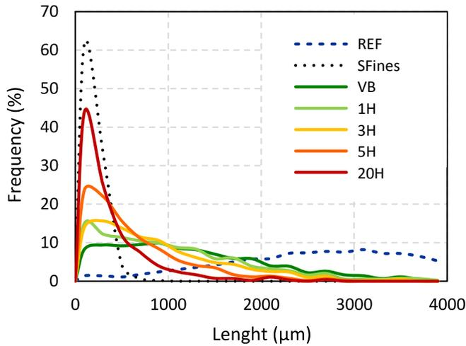
Fig. 2. Average distribution of fibre length (weight weighted) of used fibrous materials
