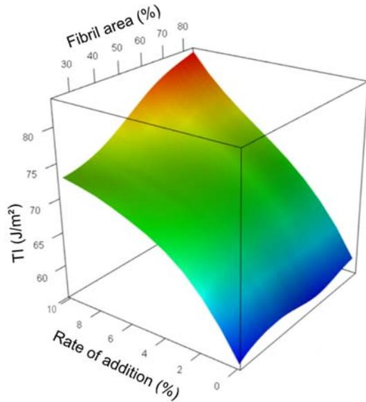
Fig. 8. Combined influence of the morphological characteristics (fibril area) of the added materials and rate of addition on tensile index (TI).
