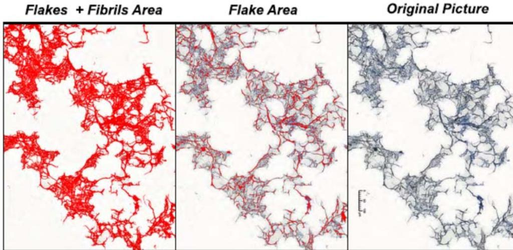
Fig. 1. Example for the result of image analysis using ImageJ Software to identify Flakes and Total detected Area in one of the 800 images realized per samples, sample 20H
