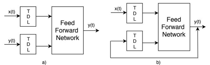
Fig. 1: Architecture of the NARX model: a) Series-parallel architecture b) Parallel architecture
