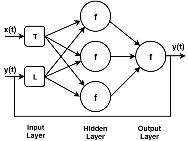
Fig. 2: Sample architecture of NARX model; inputs: temperature (T) & previous loads (L)
