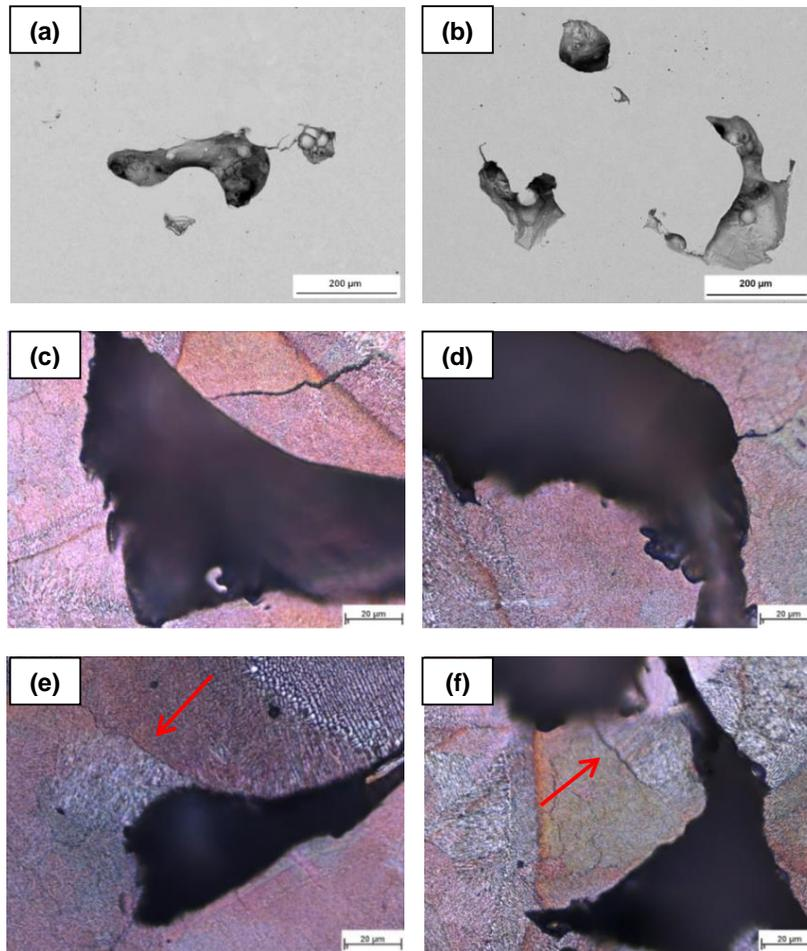
Figure 5 Pores and crack origination presented by: (a-b): SEM (BSE-mode) images; (c-d): LOM images of TMF tested samples.
