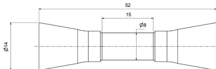
Figure 1 Sketch of TMF test specimen (in mm).
