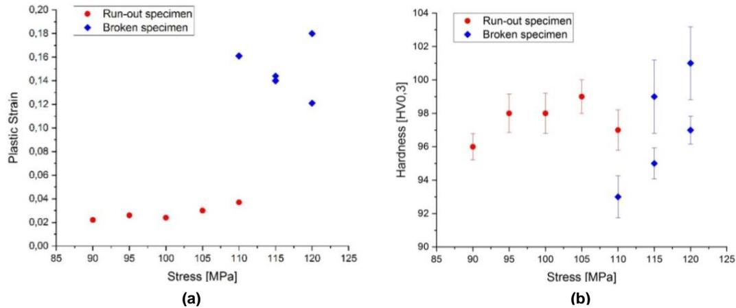
Figure 3 (a) Plastic strain due to TMF test vs. stress, (b) Hardness values with standard error after TMF tests vs. stress.
