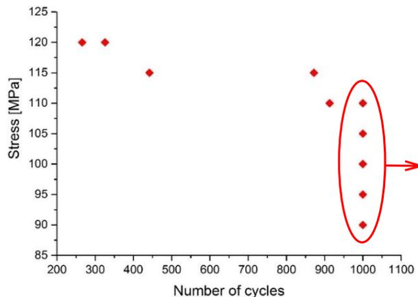
Figure 2 TMF lifetime of the samples with respect to the stress.
