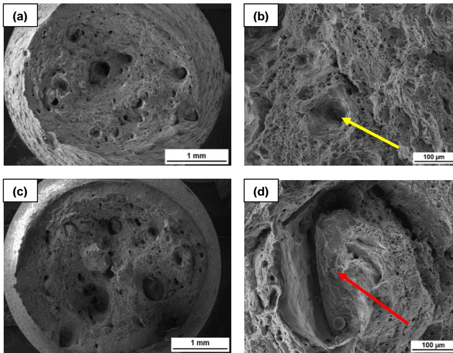
Figure 4 Fracture surface morphology of TMF test specimens under the stress of: (a) and (b) 120MPa, (c) and (d) 115MPa (Figures 4b and 4d illustrate magnified SEM images of Figures 4a and 4c, respectively).
