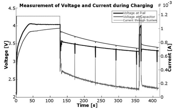
Figure 4: Measurement of the charging of prototype A.
