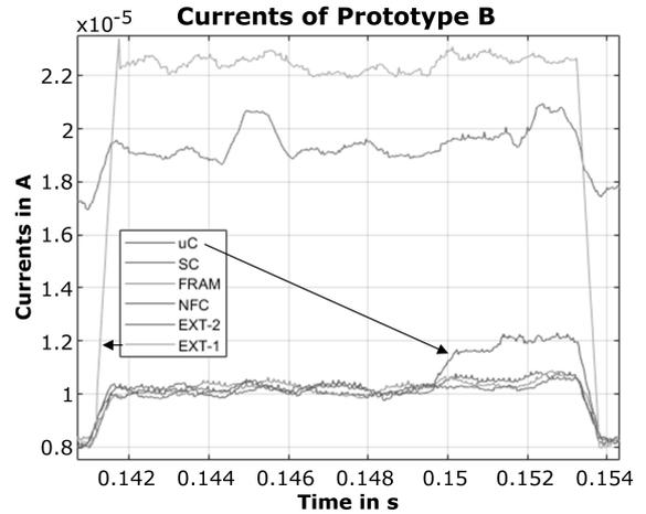
Figure 5: Current flow during measurements at prototype B.
