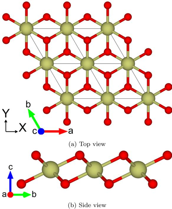
FIG. 1.  $1T$   $\text{IrO}_2$  polytype crystal structure: dark-gray (red) are oxygen atoms, light-gray (green) are iridium atoms; (a) top view, (b) side view. The  $X, Y$  axes indicate the global  $(XYZ)$  coordinate system.
