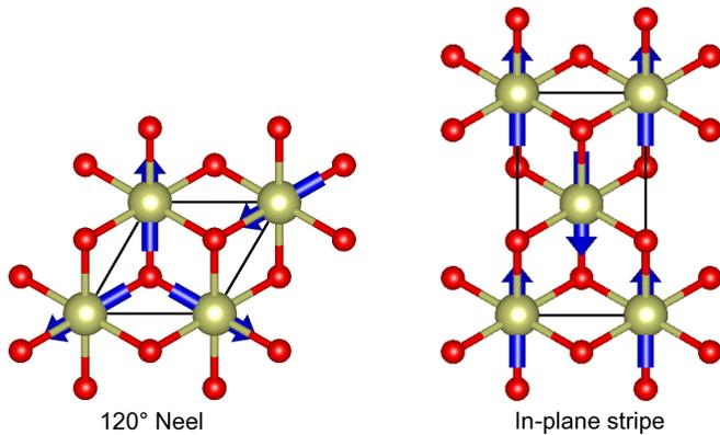
FIG. 2. The two nearly degenerate  $1T$   $\text{IrO}_2$  magnetic configurations, which are lowest in energy. The arrows show the directions of the spin magnetic moments on the Ir atoms in the  $XY$  plane.
