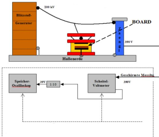
Figure 2: Test arrangement
