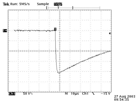
Figure 4: lightning impulse with pre-breakdown
