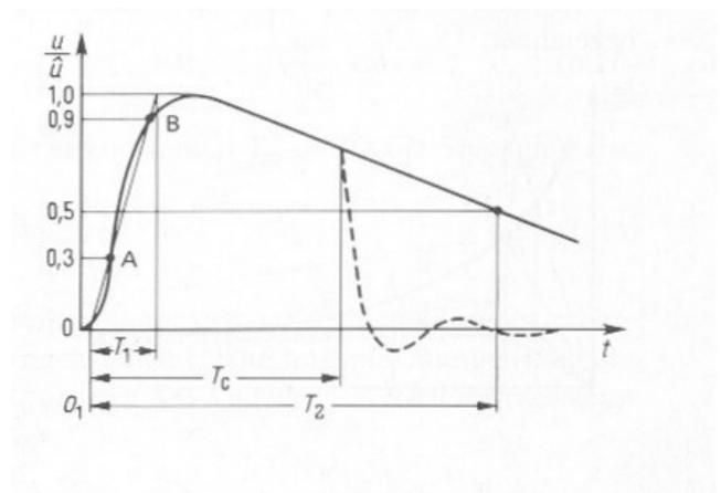
Figure 1: positive impulse voltage with the qualifying parameters
