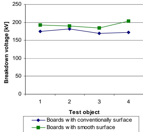
Figure 9: breakdown voltage of board specimen
