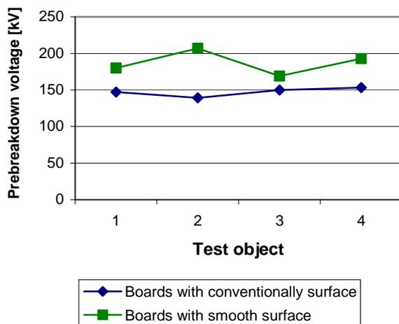
Figure 8: pre-breakdown onset voltage of board specimen
