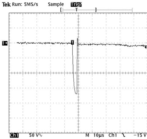
Figure 7: lightning impulse with breakdown
