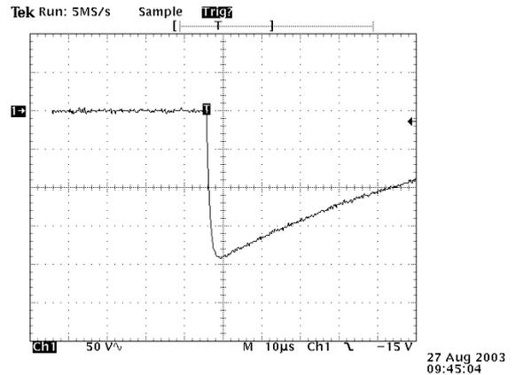
Figure 3: lightning impulse without pre-breakdown
