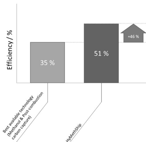
Fig. 2 Efficiency estimation for best available technology (methanol & post-combustion carbon capture) vs. HyMethShip (pre-combustion carbon capture)
