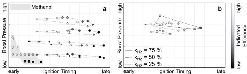
Fig. 7: Operating ranges for methanol and hydrogen operation (a) and dual fuel operation (b)
