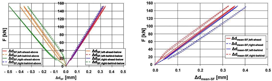
Fig. 7: Bending test diagrams: measurement of extensions of shear-field diagonals in relationship to applied force (applied force corresponds to 50 % of estimated  $F_{max,mean,est}$ ) – elongation of each shear-field diagonal measurement (left), mean elongation of each shear-field diagonal (right)
