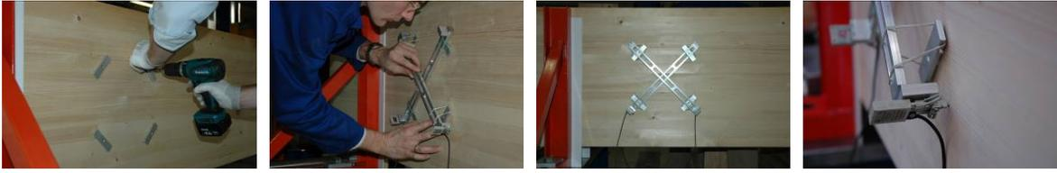
Fig. 3: Application of shear fields of series **GLT-II** and **GLT-III**: fixing of holders for rubber bands (left), mounting of measurement device (left-middle), overview (middle-right), detail of distortion measurement device DD1 with metering needle placed on a nail-head (right)
