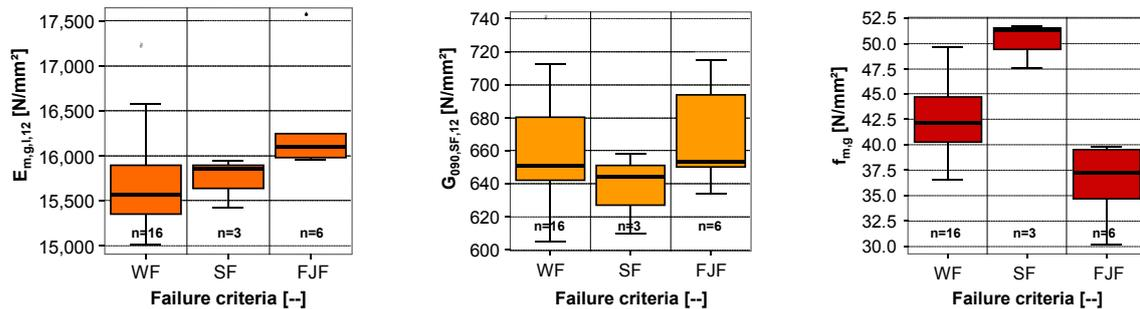
Fig. 9: Box-plots of series **GLT-II** – GL36h: according failure criteria grouped mechanical properties: local bending E-modulus  $E_{m,g,l,12}$  (left), shear modulus  $G_{090,SF,12}$  (middle) and bending strength  $f_{m,g}$  (right)
