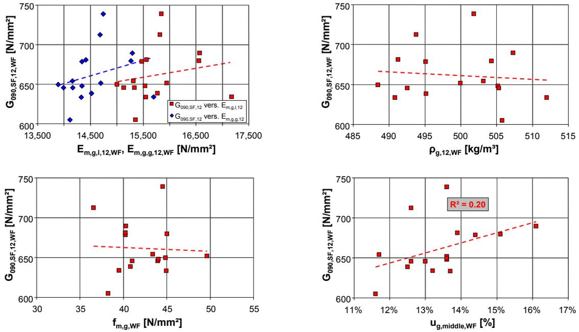
Fig. 10:  $G_{090,SF,12,WF}$  vers.  $E_{m,g,l,12,WF}$ ,  $E_{m,g,g,12,WF}$  (left-above), vers.  $\rho_{g,12,WF}$  (right-above), vers.  $f_{m,g,WF}$  (left-below) and vers. moisture in the middle of beam-depth  $u_{g,middle,WF}$  (right-below) – series GLT-II / WF
