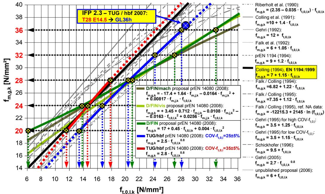
Fig. 5: ‘Bearing models for GLT in bending’ – sub-model concerning the requirements on boards – relationship  $f_{m,g,k}$  vers.  $f_{t,0,1,k}$ : past models in comparison with current bearing models for prEN 14080 and the test result of series GLT-II of GL36h (see Brandner and Schickhofer (2008))
