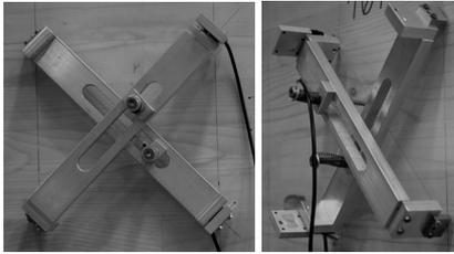
Fig. 6: Shear field test configuration of series **GLT-I** with  $L = 160$  mm
