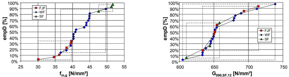
Fig. 8: Empirical distribution of the bending strength  $f_{m,g}$  (left) and shear-modulus  $G_{090,SF,12}$  (right) of series **GLT-II** – GL36h: classified failure criterias – wood failure in bending (WF), failure in the finger joint (FJF) and wood failure in shear (SF)
