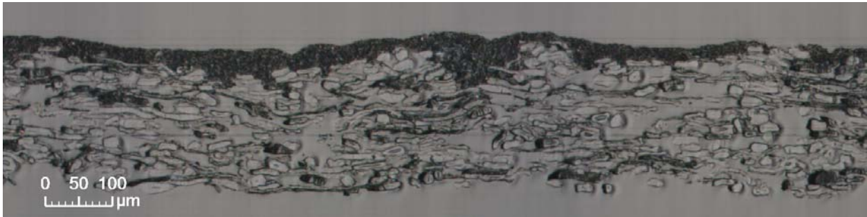
(c) Only carbonate containing coating color, low base paper porosity.
