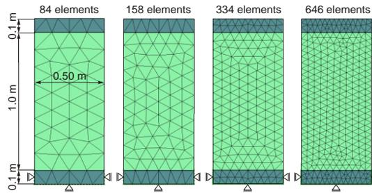
Figure 5: Numerical biaxial model and FE-meshes
