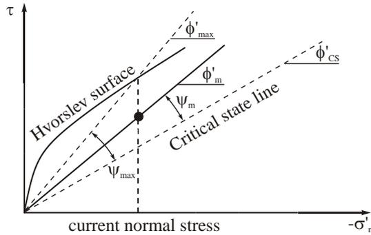
Figure 3: Mobilized and maximum angle of dilatancy
