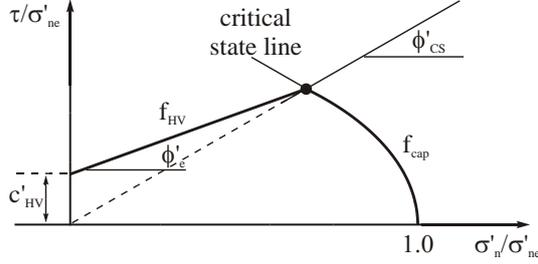
Figure 2: Local normalized shear strength envelope
