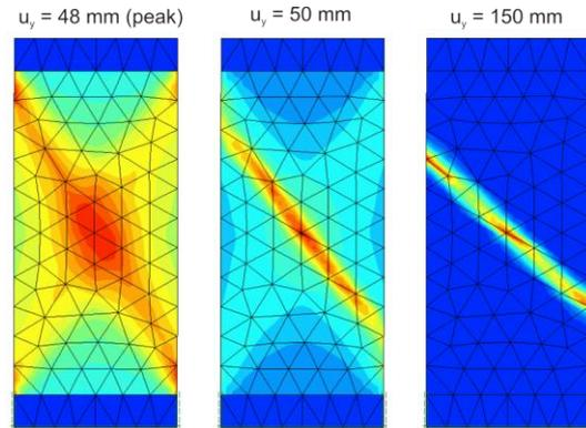
Figure 8: Shear band evolution with modified model (158 elements)
