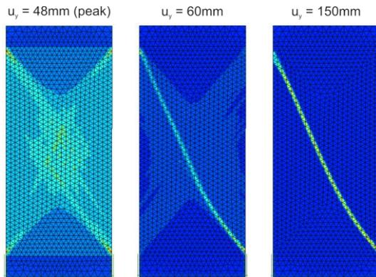
Figure 9: Shear band evolution with modified model for  $l_{cat} = 1$  cm,  $h_{soft} = 3$  (2440 elements)
