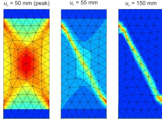
Figure 7: Shear band evolution with reference model (158 elements)
