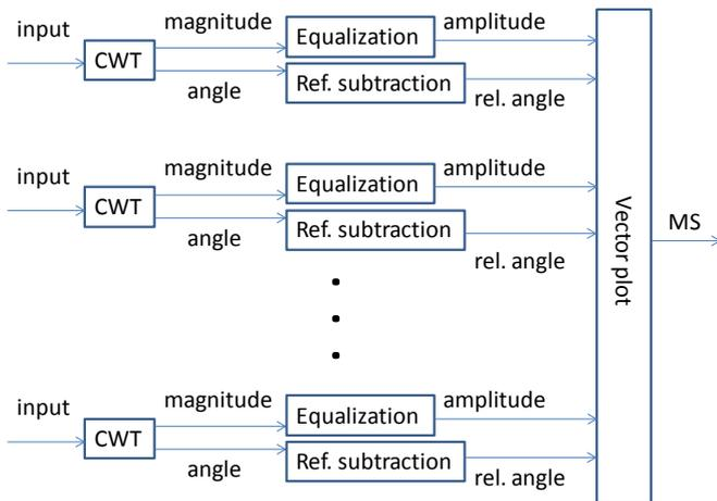
Fig. 1. Block diagram of the mode shape estimation. Input is the measured signal, e.g. voltage angle difference, CWT = continuous wavelet transform, MS = Mode Shape, rel. angle = relative angle.
