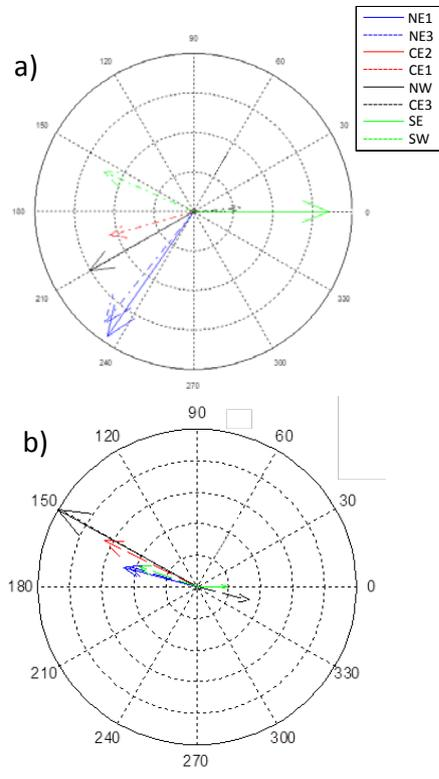
Fig. 10. Estimates of the 0.85 Hz (East-West) mode shape, voltage reference angle in location CE2. a) measurement-based estimate, b) estimate based on a detailed simulation model.
