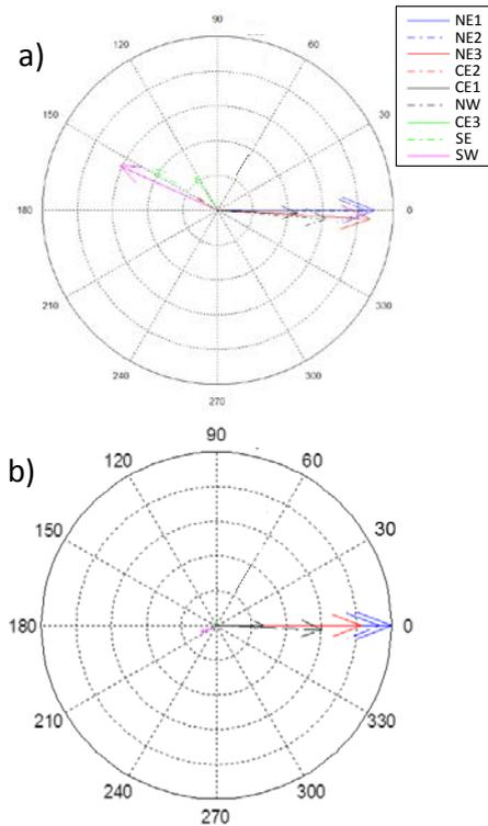
Fig. 9. Estimates of the 0.5Hz (North-South) mode shape, voltage reference angle in location CE2. a) measurement-based estimate, b) estimate based on a detailed simulation model.
