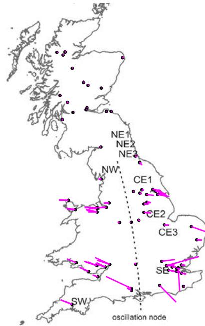
Fig. 4. Simulation-based East-West mode shape with rotor angle signals.
