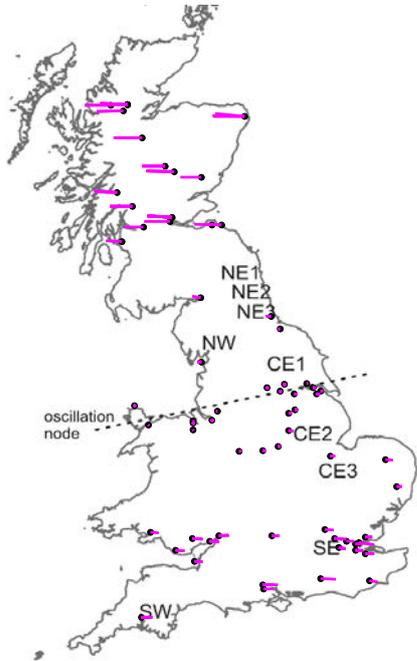
Fig. 2. Simulation-based England-Scotland mode shape with rotor angle signals.
