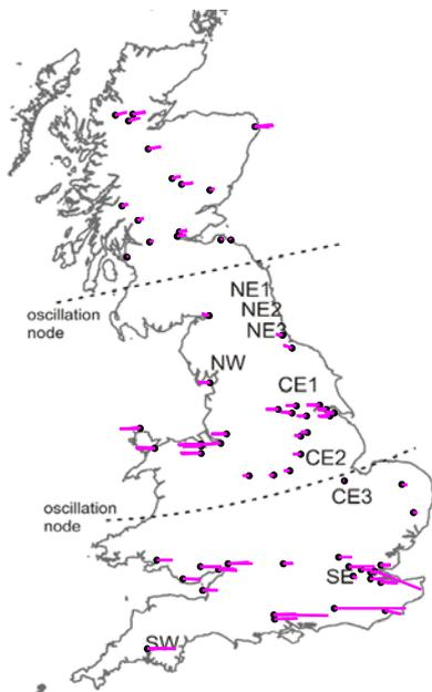
Fig. 3. Simulation-based North-South-2 mode shape with rotor angle signals.
