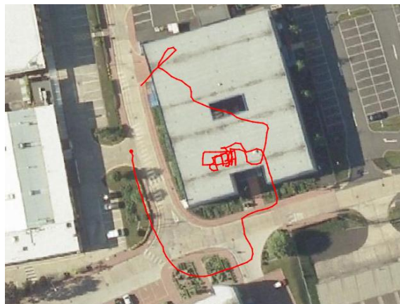
Figure 2a: Indoor navigation track with original sensor Kalman Filter
