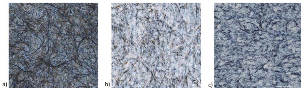
Figure 1. a) The standard Burnout- Test [3] applied to a TMP handsheet. The fibers are not sufficiently blackened. b) Standard Burnout test [3], wood fibers carbonized incompletely. c) Result of the new Burnout Test, all fibers are entirely and evenly blackened.
