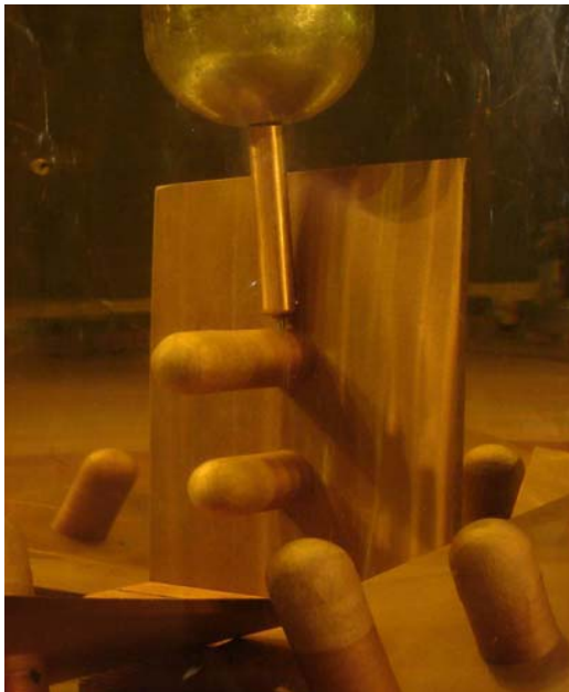
Figure 6: Test arrangement for an oil/board insulation system with two insulated electrodes, the upper electrode is on HV, the lower one is grounded
