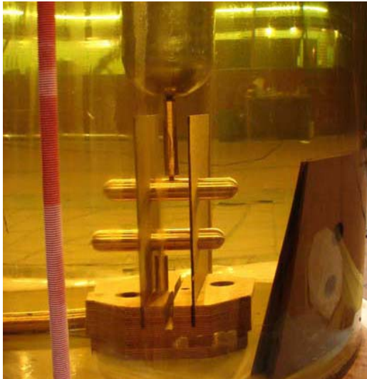
Figure 5: Test arrangement for an oil/board insulation system with two bare electrodes, the upper electrode is on HV, the lower one is grounded
