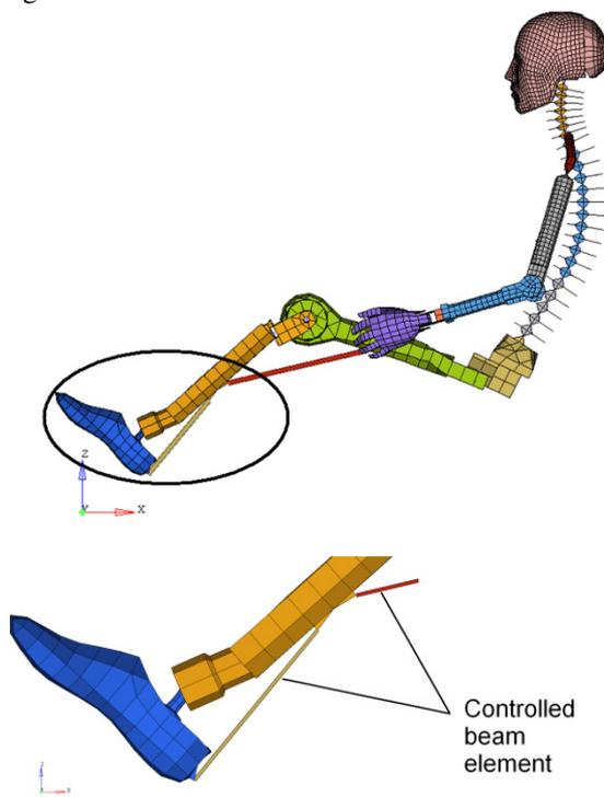
**Figure 4. Model consisting of BIORID II and H3 dummy parts, detail muscle implementation**
