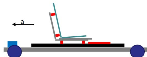
**Figure 1. Principle sled test setup. Symbol a is the sled acceleration during the test.**
