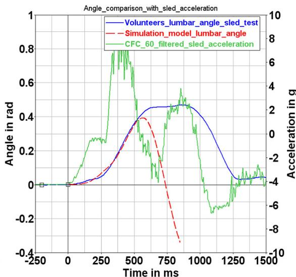
Figure 9. Sled test acceleration and volunteer lumbar angle in during sled test and simulation
