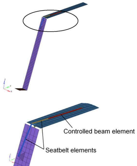
**Figure 3. Leg model substitute, detail muscle modeling with seatbelt elements and controlled beam element**
