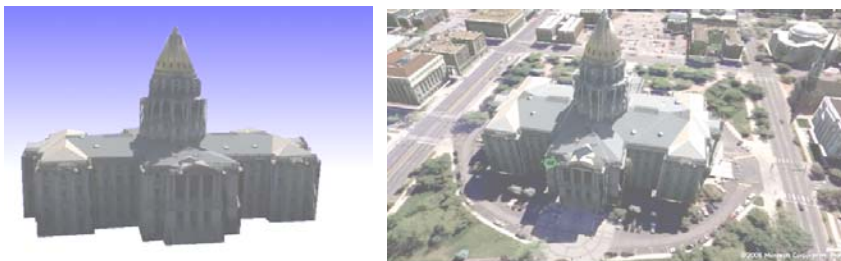
Fig. 2: A state-of-the-art automated urban model with building and terrain model as separate objects (© Microsoft ). The object shown is the Colorado Capitol in Denver, USA.
