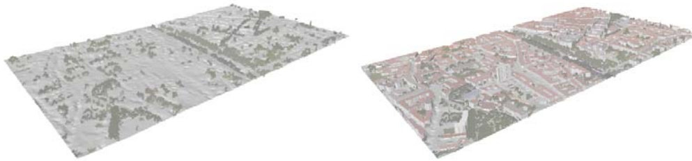
Fig. 9: A virtual 3D model of the center of Graz, Austria is generated by taking into account the semantic classification and the available 3D height information. The model on the left presents the raw DTM and the class “tree”, each tree being modeled as an individual point cloud. The right model includes the extracted building blocks, assigning to each block a mean color and height.
