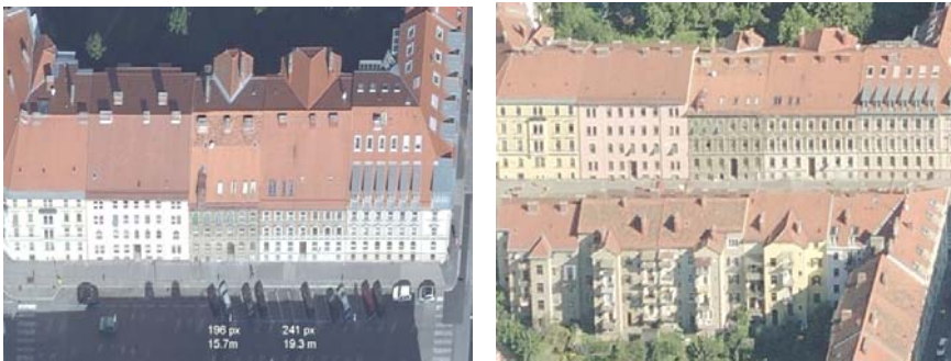
Fig. 3: View of facades, once from a tilted aerial camera (left), once from vertical aerial imagery ( Microsoft UltraCam ), but taken from the edge of such photographs.
