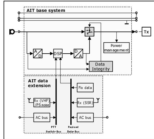
Figure 2. AIT aircraft system architecture.
