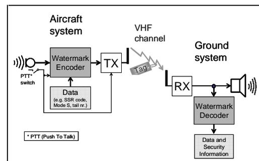
Figure 1. Voice communication link with embedded data.
