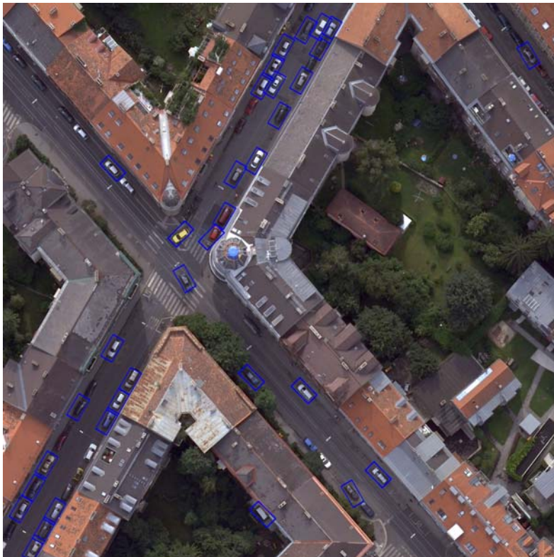
Figure 5, Visual detection results on a Graz data set scene. The blue rectangles indicate a true positive car detection.
