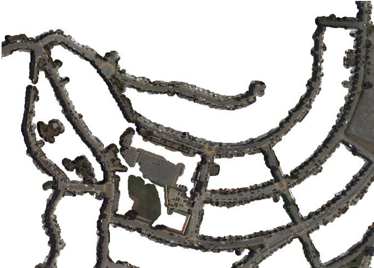
Figure 4, Extracted street layer using the interpolated DTM and color models of a San Francisco scene.
