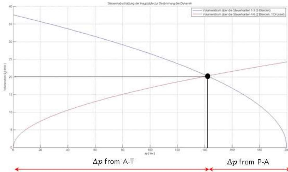
Figure 5: Analytic calculation of the volume flow through the pilot stage
