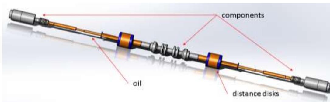
Figure 3: Modell to calculate the eigenfrequency
