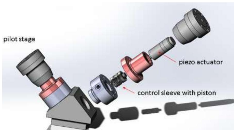
Figure 2: The two pilot stages which are mounted on the main stage
