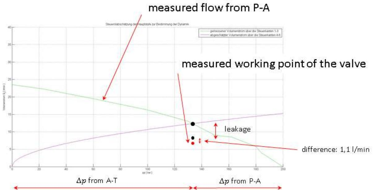
Figure 6: Measured volume flow through the pilot stage
