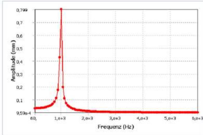
Figure 4: Eigenfrequency of the whole valve
