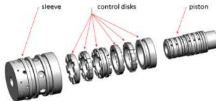
Figure 1: pilot stage (piston and control sleeve)
