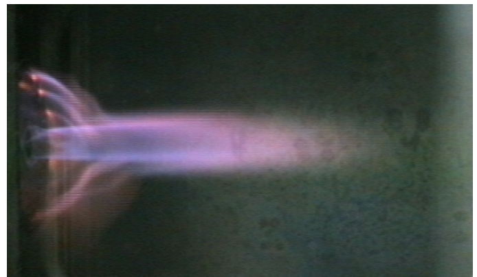
FIGURE 11. Picture of the hydrogen flame made with a CCD camera. Air and fuel inlets can be seen on the left side of the picture. The viewing direction is not perpendicular to the window.
