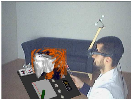
(b) Volume Rendering - The transfer function can directly be drawn onto the personal interaction panel (PIP).
